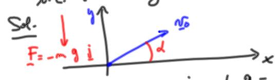
$$\underline{F} = m \underline{a} = -mg \underline{j} \quad | \quad g = 9.81 \text{ m/sec}^2$$
