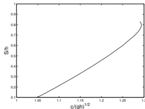
**Figure:** (a) Solitary waves of height  $S/h = 0.1, 0.3, 0.5, 0.8$ . (b) Bifurcation diagram. Computed by the modified Tanaka's method.
