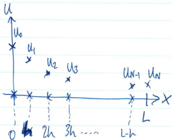
General idea: Convert the BVP into a system of algebraic equations (which we know how to solve), by replacing derivatives with finite differences. E.g.
