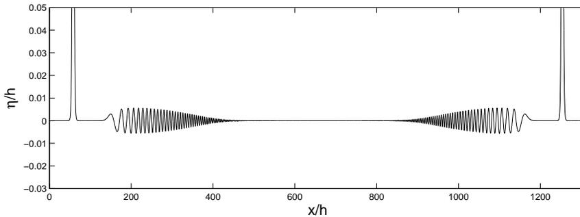
Figure 4. Results of the collision of two solitary waves of equal height  $S/h = 0.4$  after the collision at time  $t/\sqrt{h/g} = 780$ . The residual has a characteristic tear-shaped envelope
