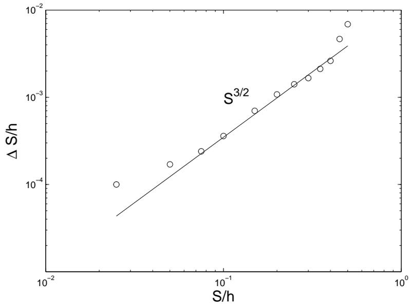
Figure 8. Change in amplitude  $\Delta S/h = (S - S^+)/h$  vs. wave amplitude  $S/h$ : numerical results (circles), power law  $(S/h)^{3/2}$  (solid line).
