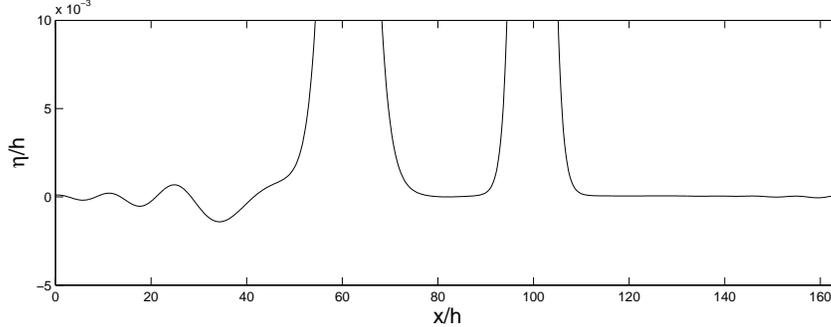
Figure 6. Overtaking collision of two solitary waves of height  $S_1/h = 0.4$ ,  $S_2/h = 0.1$  at  $t/\sqrt{h/g} = 745$ , which is after the collision. The vertical scale is magnified in order to observe the dispersive trailing wave generated by the interaction.
