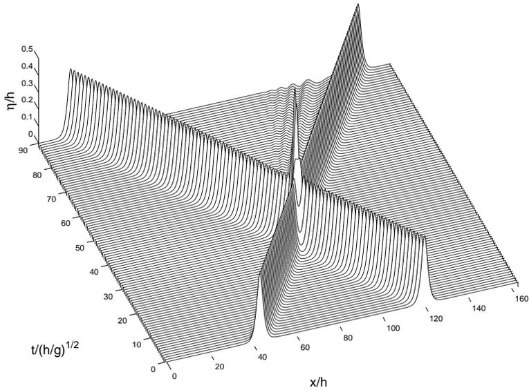
Figure 2. Head-on collision of two solitary waves of equal height  $S/h = 0.4$ : The amplitude after collision is  $S^+/h = 0.3976$  at  $t/\sqrt{h/g} = 90$ . The phase lag is  $(a_j - a_j^+)/h = 0.3257$ .
