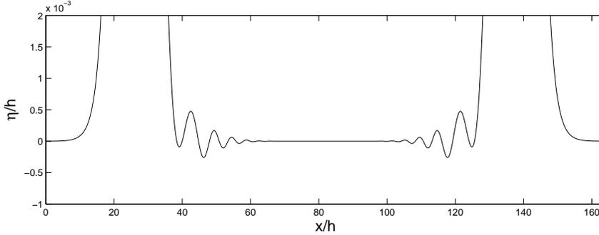
Figure 3. Results of the collision of two solitary waves of equal height  $S/h = 0.1$  after the collision, at time  $t/\sqrt{h/g} = 90$ . The dispersive residual wave trailing the solitary waves after the collision are visible under magnification.
