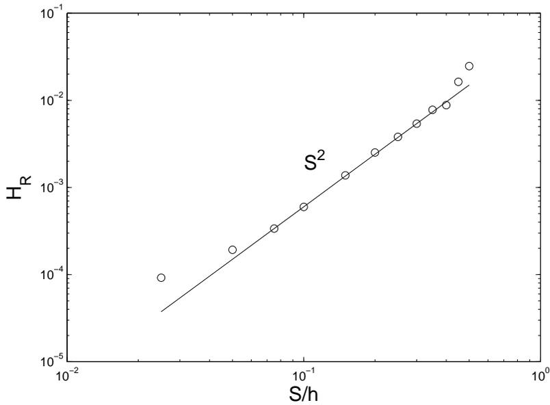
Figure 9. Energy of the residual  $e_R$  vs. nondimensional wave amplitude  $S/h$ : numerical results (circles), power law  $(S/h)^2$  (solid line).
