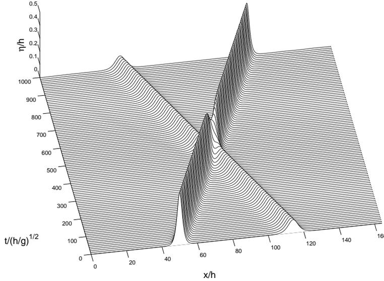
Figure 5. Overtaking collision of two solitary waves of height  $S_1/h = 0.4$ ,  $S_2/h = 0.1$ : The amplitudes after collision are  $S_1^+/h = 0.4003$ ,  $S_2^+/h = 0.0999$  at  $t/\sqrt{h/g} = 1000$  for the large, small wave respectively. The phase shifts are  $(a_1^+ - a_1)/h = 2.2974$ ,  $(a_2^+ - a_2)/h = 3.6159$  respectively.
