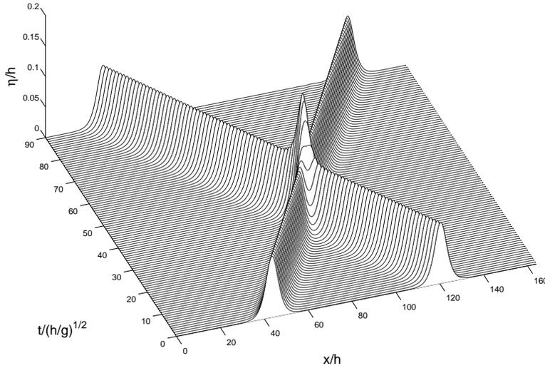
Figure 1. Head-on collision of two solitary waves of equal height  $S/h = 0.1$ : The amplitude after collision is  $S^+/h = 0.0997$  at  $t/\sqrt{h/g} = 90$ . The phase lag is  $(a_j - a_j^+)/h = 0.1370$ .
