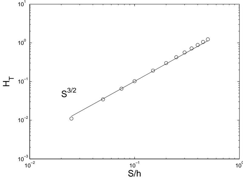
Figure 7. Total energy  $E_T$  vs. wave amplitude  $S/h$ : numerical results (circles), power law  $(S/h)^{3/2}$  (solid line).
