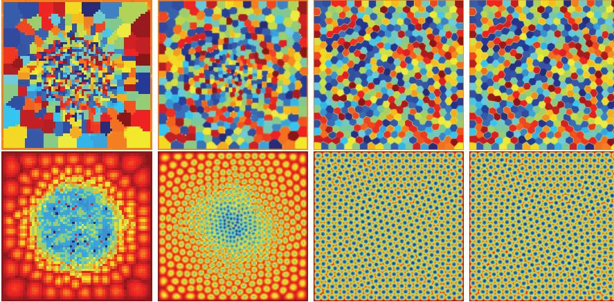
FIG. 3.7. Optimization of the sum of the first eigenvalue of the Dirichlet–Laplacian of 512 cells with  $C = 10^5$ . First row: cell shape on recursively refined grids  $(64 \times 64)$ ,  $(127 \times 127)$ ,  $(253 \times 253)$ , and  $(505 \times 505)$ . Second row: sum of the first eigenvalues on the same grids.
