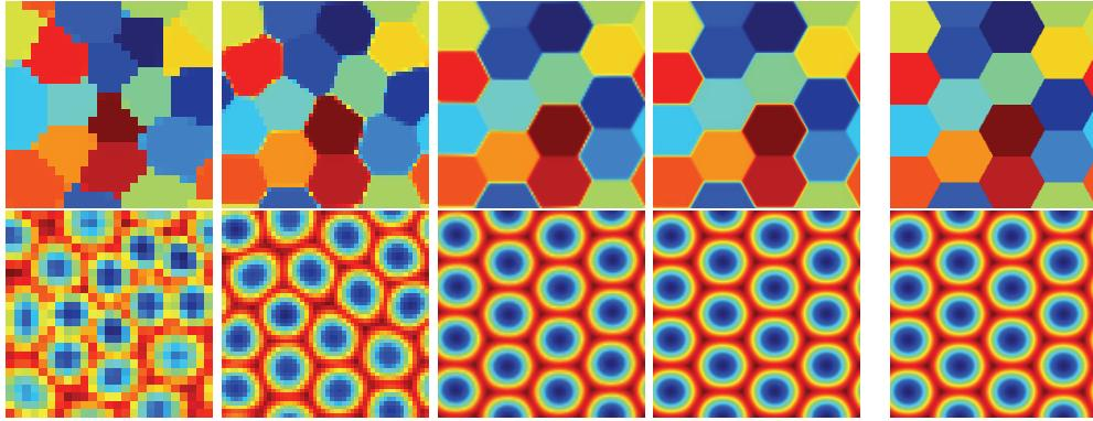
FIG. 3.4. *The same problem is solved again using the simple projection on increasingly refined grids (four leftmost figures) and then using the orthogonal projection on the final grid (right). The grid sizes are (from left to right)  $25 \times 25$ ,  $50 \times 50$ ,  $100 \times 100$ , and  $200 \times 200$ . The objective function upon convergence is (from left to right) 1,902.1, 2,033.8, 2,095.7, 2,124.6, and 2,048.8.*
