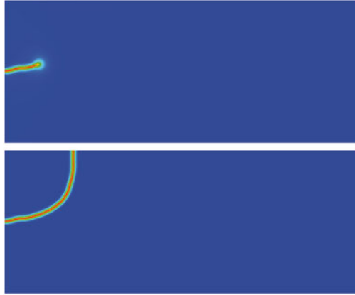
Figure 4.3.8. Position of the crack set in the tearing experiment for t = .18 (top) and t = .19 (bottom).
