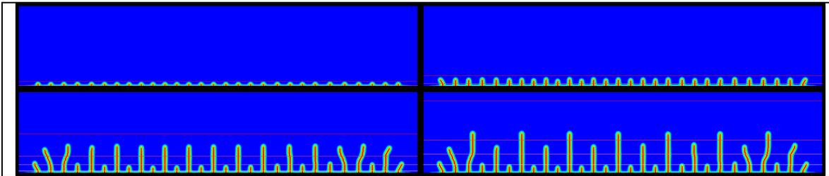
Figure 1: Convective heat transfer in a glass slab. Snapshots of the crack set and iso-temperatures at times  $t=5E-4, 2.25E-3, 2.5E-2$ , and  $8.E-2$ .
