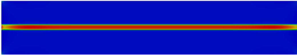
(a) High stress region in brittle layer prior to fracture formation
