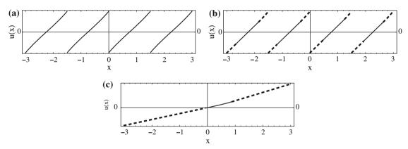
Fig. 8 The optimal displacement fields for the states A, B, C of Fig. 7. Debonded regions are indicated with a dashed line
