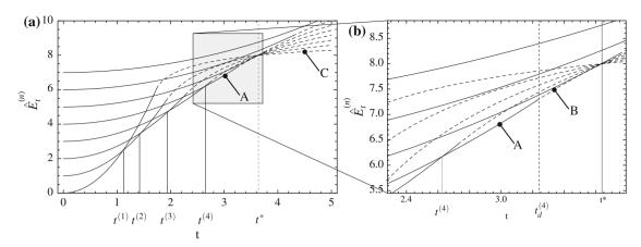
Fig. 7 Energy curves  $\hat{E}_t^{(n)}$  with possible debonding and transverse fracture for  $\gamma=2.2, L=6$ . Each curve is for a specific number n-1 of transverse fractures, corresponding to the value at the intersection with the axis t=0. The *solid continuous lines* indicate the energy is obtained for a state without debonding, the *dashed line* for a state with debonding
