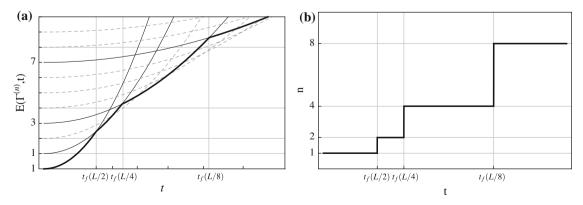
Fig. 10 Quasi-static evolution without debonding: a energy curves  $E(\Gamma^{(n)}, t)$  versus t for different n, where the thick solid line denotes the global minimum corresponding to the solution of the evolution problem; **b** number of parts  $n_j$  of length  $L/n_j$  versus t formed by the  $n_j - 1$  equally spaced cracks, with  $n_j = 2^j$
