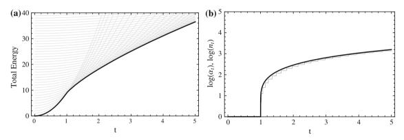
**Fig. 5** Energy and fracture density curves in the "long film" regime. *Thick lines* show the results of the limit model, they are compared with the discrete family of energies (20). The limit model can macroscopically characterize high fracture density regimes with a "damage"-like parameter
