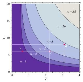
Fig. 13 Phase diagram for the coupled transverse cracking and debonding problem. For a quasi-static evolution, to each couple of parameters  $(L, \gamma)$  the phase diagram associates the (maximum) number of parts n into which the film is split before debonding takes place. We point out with a *white dot* the couple of parameters of the evolution illustrated in Sect. 5.3, with a *red dot* the couples of parameters referring to the numeric experiments detailed in Sect. 6 (color figure online)
