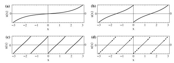
Fig. 12 Snapshots of the displacement field for states O, A, C, D of Fig. 11a. The debonded region is indicated with a thicker dashed line
