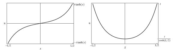
Fig. 2 Elastic displacement (left) and deformation (right) for a sound film of dimensionless length L=6
