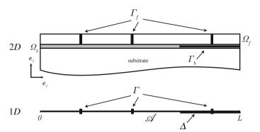
Fig. 1 2D: A cross-section of the 3D system: the film  $\Omega_f$  is bonded to a stiff substrate by the means of the bonding layer  $\Omega_b$ . Transverse cracks  $\Gamma_f$  debonding cracks  $\Gamma_b$  may develop in the film and in the bonding layer. 1D reduction: in the reduced uniaxial elastic bar of axis  $\mathscr{A}$ , transverse and debonding cracks are identified with  $\Gamma$  and  $\Delta$
