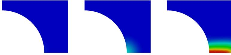
**Fig. 15.** Damage field at the boundary of the hole in the elastic phase  $0 < t < t_e$  (left), the phase with partial damage  $t_e < t < t_c$  (center), and after the nucleation of a crack  $t > t_c$  (right). Blue:  $\alpha = 0$ , red:  $\alpha = 1$ . The simulation is for  $\rho = 1.0$  and  $a/\ell = 5$ . (For interpretation of the references to colour in this figure legend, the reader is referred to the web version of this article.)
