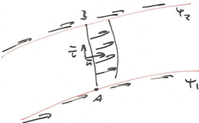
What is the volume flux between the two streamlines?
