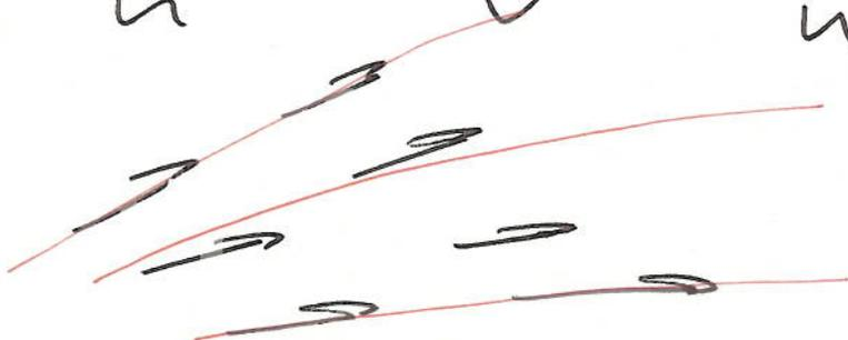
[ particle displacement  $d\vec{r} = [dx, dy, dz]$  everywhere in the direction of the velocity field ]
