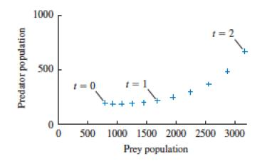
The graph of a solution in the phase plane is called a **phase-plane trajectory**.
