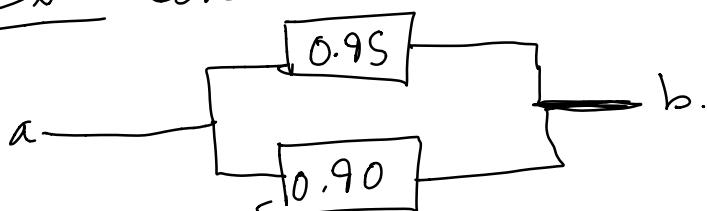
• The numbers indicate the probability that the device is functional. Assuming the devices
