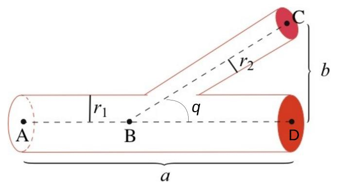
$$R(q) = C \left( \frac{a - b \cot q}{r_1^4} + \frac{b \csc q}{r_2^4} \right)$$
