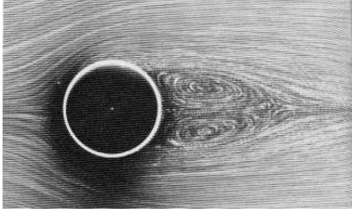
Figure 1.2: Visualisation of the cylinder flow by Taneda;  $Re = 26$ .
