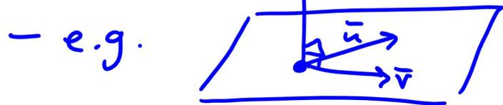
Find normal  $\bar{n}$  to plane containing  $\bar{u}, \bar{v}$
