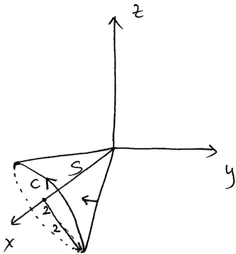
The boundary of the surface is the circle  $C$  with radius 2 in the plane  $x=2$ . The orientation of  $C$  induced by the orientation of  $S$  is counterclockwise when viewed in the negative  $x$ -axis direction. (Indicated in the above picture).
